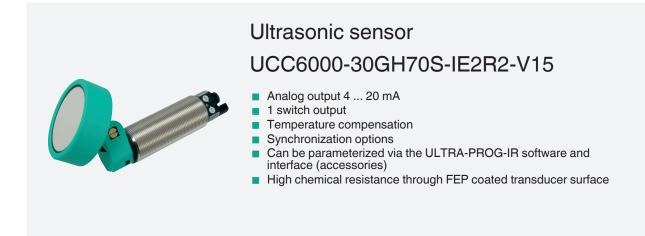
Ultrasonic diffuse sensor with pivoting transducer
