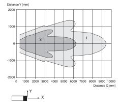
Curve 1: flat surface 100 mm x 100 mm Curve 2: round bar, Ø 25 mm Accessories
